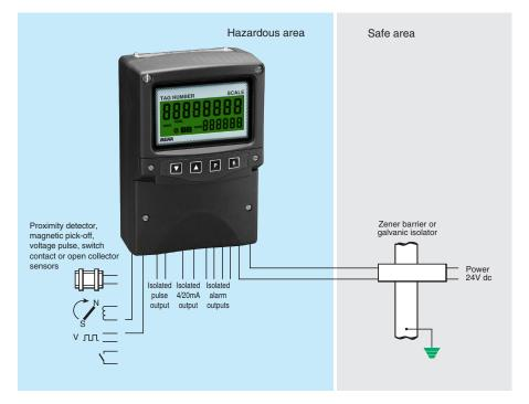
The BA334E is a third generation intrinsically safe field mounting rate totaliser housed in a robust IP66 GRP enclosure with a seperate terminal compartment. The totaliser is easy to use and can be configured on-site to operate with flowmeters having a magnetic pick-off, switch contact, proximity detector, open collector or a voltage pulse output. International intrinsic safety certification permits worldwide installation.
